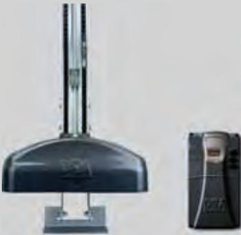
*Dea Advance 600 N Motor, maximum force 60 Kg, equipped with control panel and 433 MHz radio receiver with 2 channels, speed control system and slowing down system for opening and closing, standard sensor against finger crushing, courtesy light to light up the working area. Separate control unit with button panel, It is supplied with chain guide with a standard length of 3000 mm and 3600 mm. further extensions are available if necessary.*
